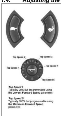
The user can adjust the wheelchair's top speed to suit their preferences and environment. The currently selected top speed is shown on the Speed indicator and can be adjusted using the "Increase Speed" (Hare) and "Decrease Speed" (Tortoise) buttons.
