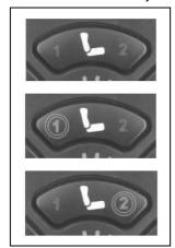
Two seat functions are available for individual adjustment and are accessed via the Seat Function Button.
